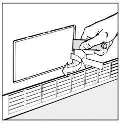
Keep hold of the outer condenser unit cover while removing it, then place it to one side.
